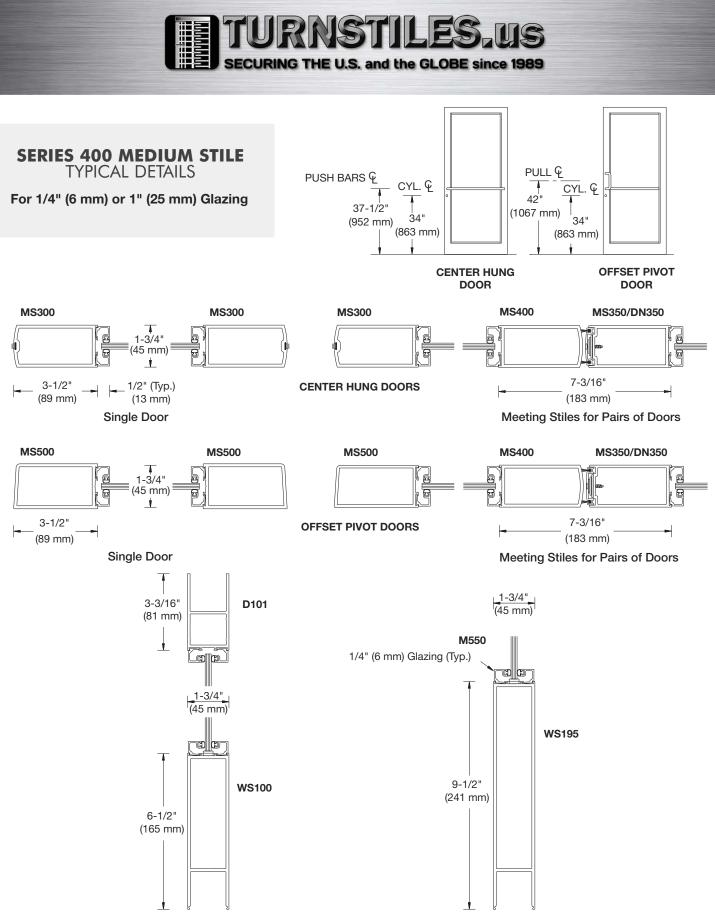
Standard Top and Bottom Rails Special Bottom Rail to Comply With A.D.A.
