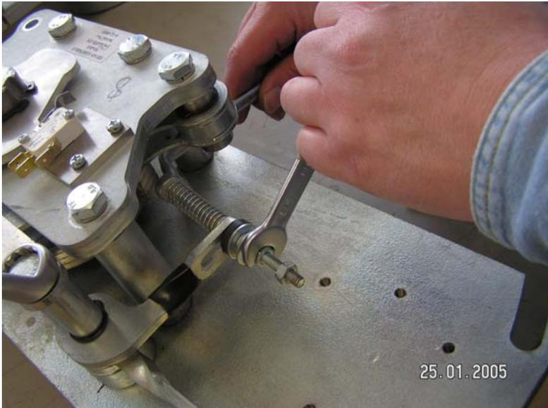
4. Remove the lever and the bolt.
