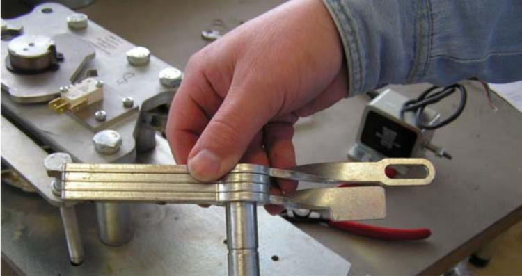
**9. Insert the circlip.**
