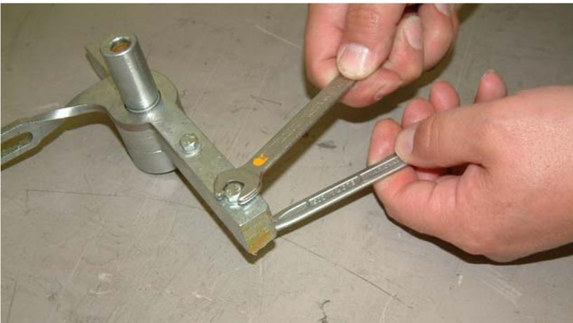
**7. Replace the new lever and connect it with the connection screws.**
