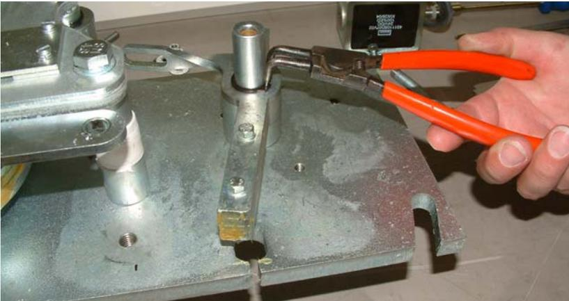
**6. Loosening of the connection screw and remove the lever according to the figure below.**
