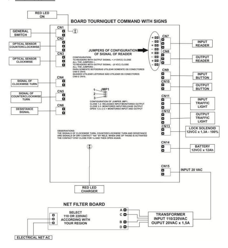
The sensor is connected according is showing in the above drawing case the entry was by right access. Case the entry access was by left, invert the position of the sensors in CN2 and CN3.
